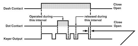
Dot contact made after dash has started but before space time has expired, will give proper dot.
