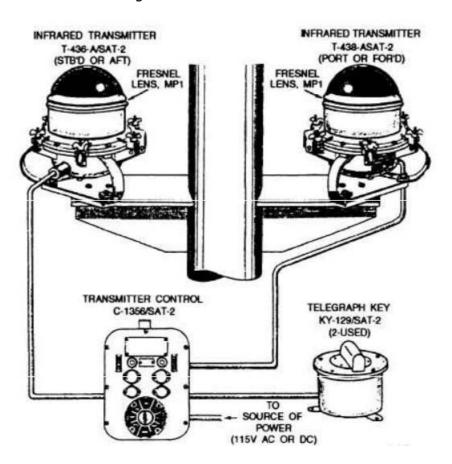
The IR transmitting set consists of two IR transmitters (beacons), a transmitter control panel, and two telegraph keys. The beacons may be operated separately or simultaneously by either manual key. Selection of the mode of operation is controlled by the transmitter control panel. The IR transmitter consists of a formed brass housing and a dome-shaped homogeneous tempered glass filter, which encloses a 300-watt, 110-volt, T20 clear bulb incandescent lamp and reflector.
