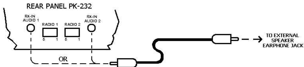
Figure 3-1 Receive audio connection to the PK-232.
