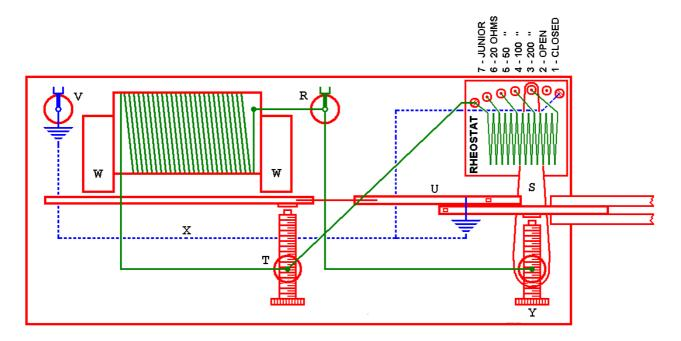
Cut No. 2 shows wiring diagram and details of rheostat and electro-magnet.
