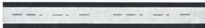
Fig. 2. Sample of tape showing signals at 20 words per minute. Tape speed 1.8 metres per minute.
