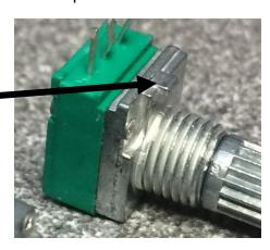
Put the volume control on to the board, it must be on the side near to the pitch control as in this picture if your fitting it into the box with the full kit.
