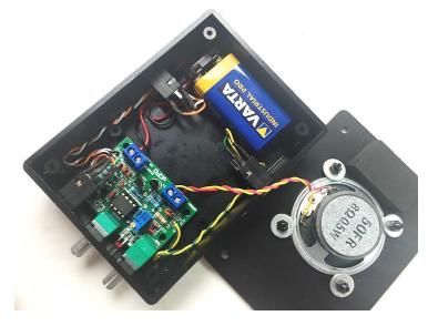
Now connect up the battery clip and speaker as shown here, the foam block is there just to stop the battery from moving around.
