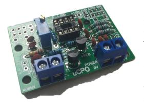
Time to take a break again and carefully check all the work you have done so far, check that all the joints are good and that you have not made any solder bridges between pins, if you have one use a maginifing glass to inspect each joint one by one. The most common reason kits don't work is poor soldering and short circuits. Make sure yours look good.
