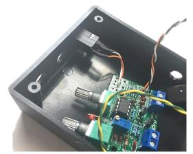
Once you have fitted the key jack then push the PCB in place making sure the LED is seated in the small hole, use the washers and nuts provide to secure the board.
