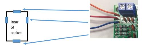
Important:- If you are not fitting the headphone socket you need to fit a link on the PCB or you will get no audio on the speaker connection block.
