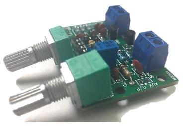
common fault with this kit is forgetting to solder the other pins of this control. Once you're happy that the control is fitted as the photo then make sure all five pins are soldered in place.
