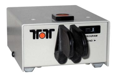
TEN-TEC Model KR1B was designed specifically for use with the Model 561 CORSAIR II transceiver. Mechanical features include a touch sensitivity adjustment and independent control of each paddle travel. A PROGRAM-SEND switch and SEND button control the built-in memory keyer in the CORSAIR II.
