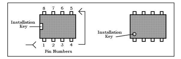
**Note:** The IC body has a small notch, or key, molded at one end, indicating pins 1 and 8. A small dimple-like body-molding is often found adjacent to pin 1. Some IC packages may include both key indicators.
