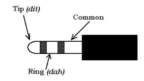
3.5 mm stereo jack. Refer to the connector packaging for wiring terminal details.
